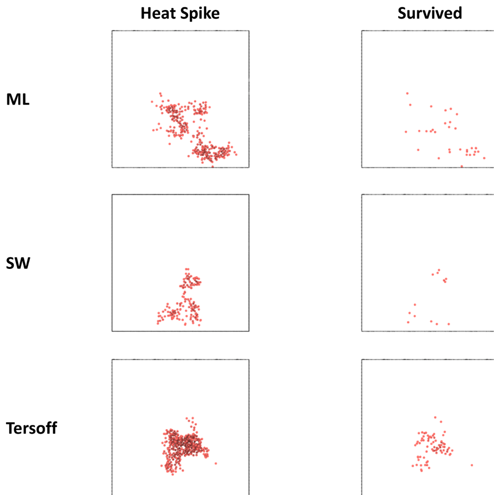
Fig. 4. Snapshots of interstitials in 1 keV PKA collision simulations at the heat spike and final stage. The ML potential produces interstitials in a larger area during the heat spike stage, eventually producing most isolated interstitials in a larger area and a few medium-sized and large interstitial clusters, which is consistent with the size distribution of interstitial clusters with ML potential in Fig. 3. The SW and Tersoff potentials produce interstitials only in a relatively small area during the heat spike stage, while only isolated and medium-sized interstitial clusters are eventually retained based on the SW potential, and Tersoff potential produced large interstitial clusters and a few medium and small interstitial clusters, which is also consistent with the size distribution of interstitial clusters with SW and Tersoff potentials in Fig. 3. Interstitials were obtained by Wigner-Seitz analysis.
